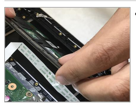
Lift the trackpad up from the laptop and slide it out of the housing.
