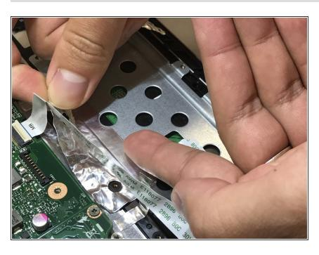
Remove all of the metallic tape holding the metal bracket to the components surrounding it.
