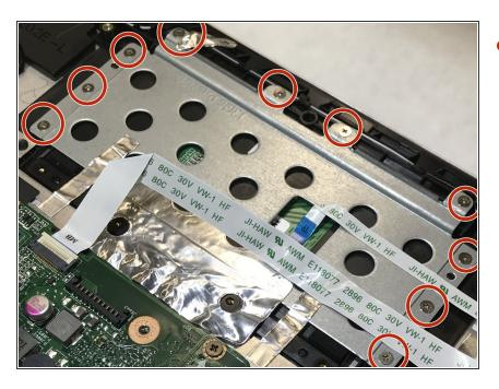
Identify the ten 2.94mm screws on the metal bracket.
