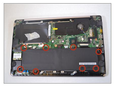
Remove the eight 4.7mm Philips #00 screws holding the battery in place.
