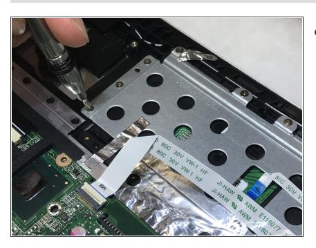
Unscrew the ten 2.94mm screws with the Philips #00 Head.
