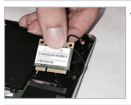
Pull the wireless card from connector slot.
