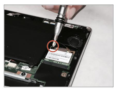
Remove the one 4.9mm screw that holds the wireless card in place with a Phillips #00 screwdriver.
