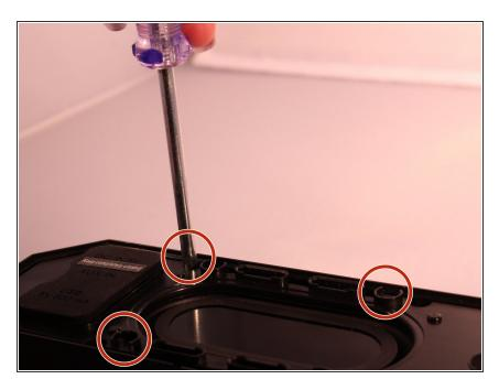
Using the size PH1 screwdriver remove the screws exposed from the rubber stoppers (4 + 2).
