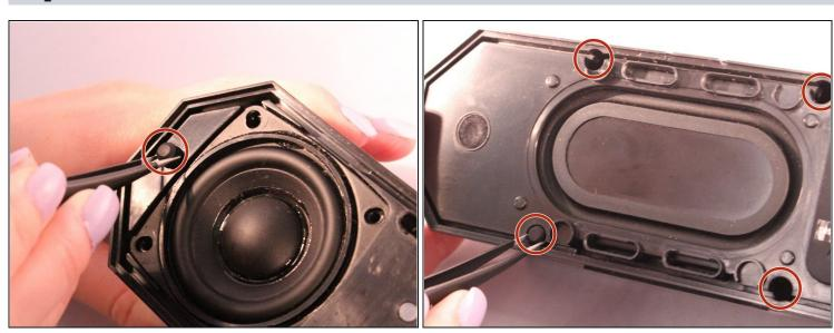
Using tweezers remove the rubber stoppers (4 at the back + 2 at the front).
