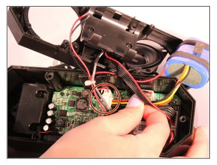
Unplug and disconnect the battery from the motherboard.
