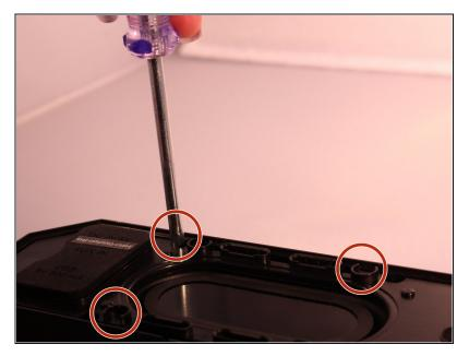
Using the size PH1 screwdriver remove the screws exposed from the rubber stoppers (4 + 2).
