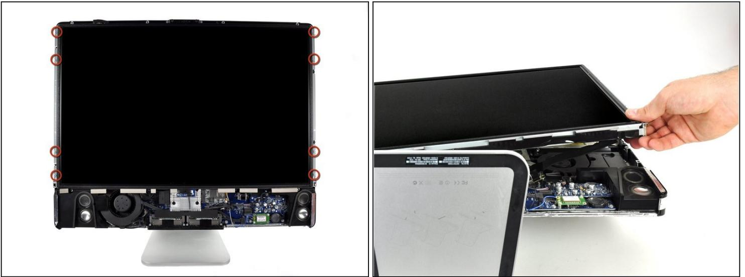
**⚠ Lay the iMac down on a table before you remove the LCD so that it doesn't fall.**
