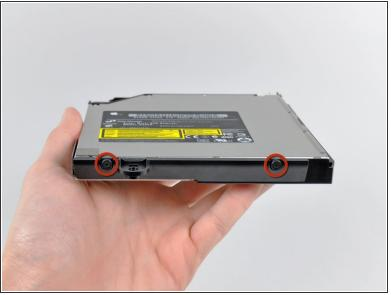
Remove the two 6.3 mm T6 Torx screws securing both sides of the optical drive bracket to the optical drive (four screws total).
