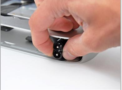
Rotate the AC-In connector 90 degrees counter-clockwise.
