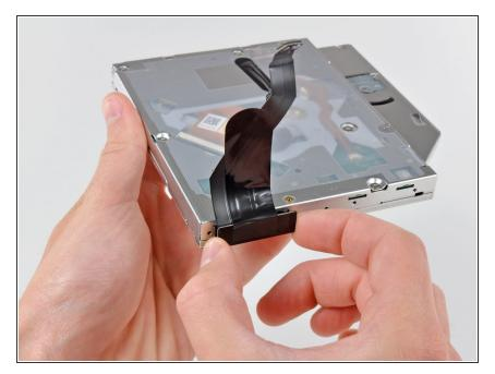
Disconnect the optical drive cable by pulling its connector away from the body of the optical drive.
