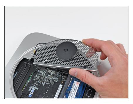
Remove the antenna plate from the mini.
