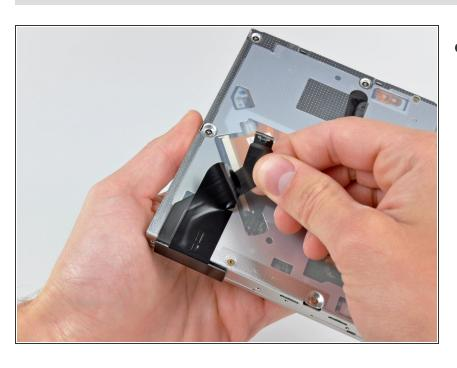
Carefully peel the optical drive ribbon cable off the body of the optical drive.
