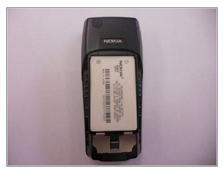
Start by taking off the back, so that you expose the back of the phone/battery like this.
