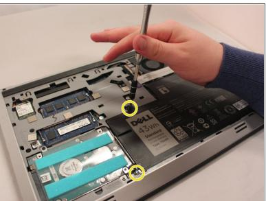
Remove the two 5.70mm Phillips #0 screws that secure the battery in place on its left side.
