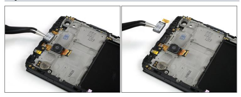
• Use a pair of <u>tweezers</u> to carefully lift the earpiece speaker out of the device and remove it.
