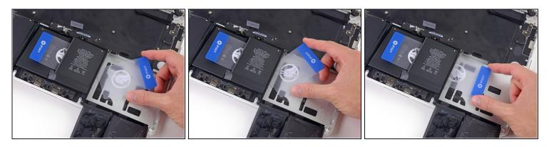
• Push one corner of a plastic card below the plastic battery frame and underneath the remaining adhered edge of the lower center cell.
