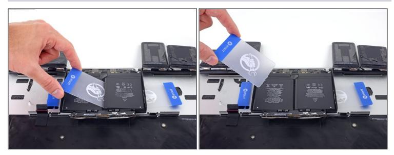
• Remove the first card that you inserted under the final battery cell.
