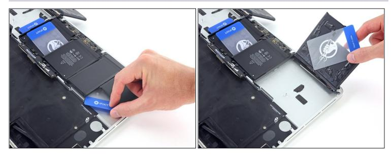
• If you haven't already done so, lift and flip the two outer left battery cells to clear access to the outside edge of the final battery cell.
