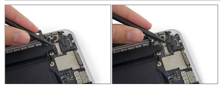
• Use the tip of a spudger to flip up the display data cable lock and rotate it toward the MagSafe 2 power port side of the computer.
