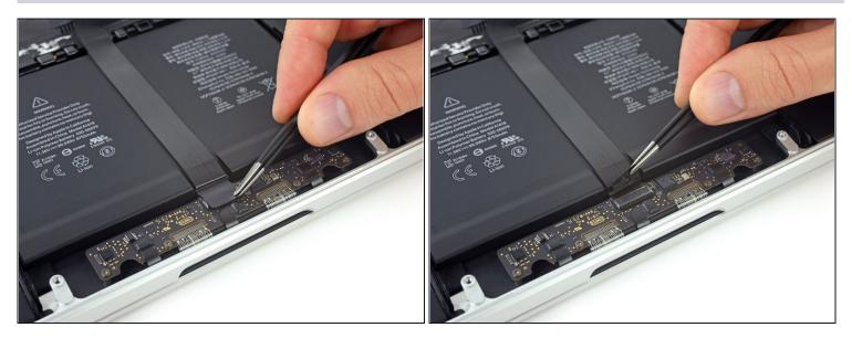
• Peel back the tape covering the trackpad connector ribbon cable, near the front edge of the MacBook Pro.
