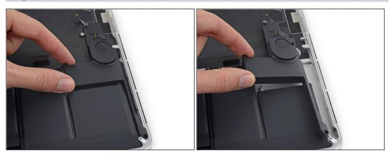
• Remove the left speaker by pulling it slightly away from the side of the upper case, and out from under the aluminum tab blocking it in.
