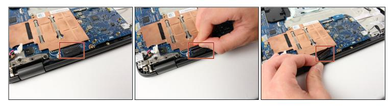
• Lift black clasp and gently pull on the back of the wire until it completely disconnects from the motherboard.
