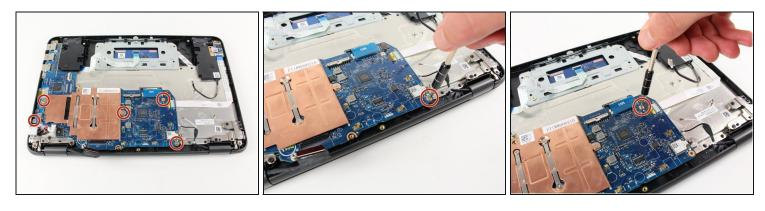
Using a Phillips #0 screwdriver, remove the five 3mm screws.
