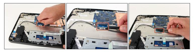
• Lift the black clasp and use the spudger tool to remove the ribbon so that it completely disconnects from the motherboard.
