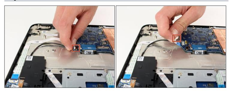
• Locate and gently pull the wire harness (small plastic box with wires leading to the black audio speakers) directly out of the connector on the motherboard.
