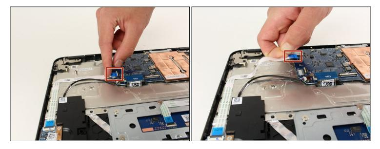
• Lift the black clasp and gently pull on blue ribbon until it completely disconnects from the motherboard.
