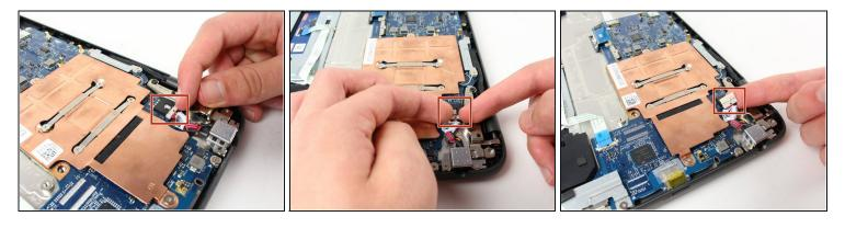
• Locate and gently pull the wire harness (small plastic box with two pink, one orange, and two black wires) directly out of the connector on the motherboard.
