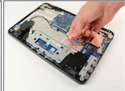
• Lift the black clasp and gently pull on blue ribbon until it completely disconnects from the motherboard.
