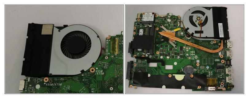
Turn the motherboard over so that the copper heat sink and fan pin connections are facing towards you.
