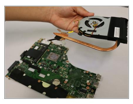
• Remove the fan assembly from the motherboard.
