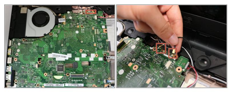
Lift the black and white wires out of their ports at the top of the motherboard.
