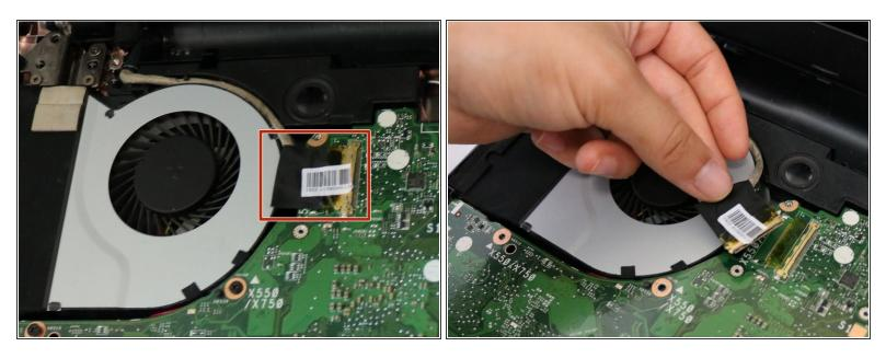
• Gently pull the thick wire in between the fan and the motherboard. To release the wire connected to the motherboard, gently pull towards the cooling fan.
