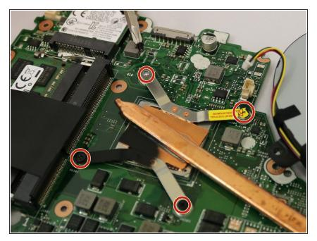
• Remove the four 4mm Phillips #0 screws that are binding the copper heat sink to the motherboard.
