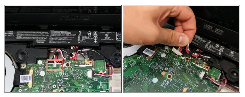
Disconnect the multi-wire battery plug from the motherboard.
