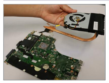
Remove the fan assembly from the motherboard.
