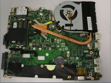
• Turn the motherboard over so that the copper heat sink and fan pin connections are facing towards you.
