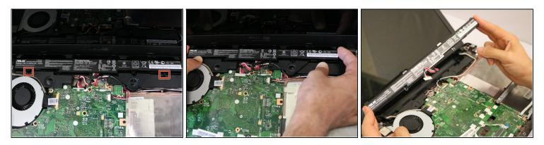
• Pull the two tabs holding the battery in place and lift the battery up. It should remove easily.
