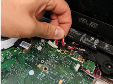
Disconnect the multi-wire battery plug from the motherboard.
