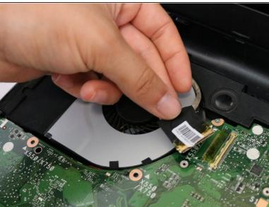
Gently pull the thick wire in between the fan and the motherboard. To release the wire connected
