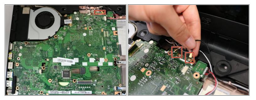
Lift the black and white wires out of their ports at the top of the motherboard.
