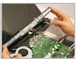
• Pull the two tabs holding the battery in place and lift the battery up. It should remove easily.
