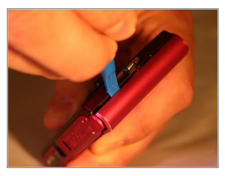
Using the plastic opening tool, separate the edge-casing from the rest of the camera.
