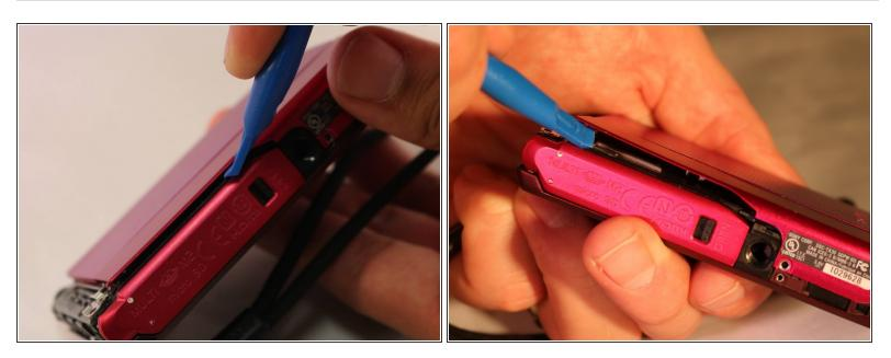
Using the plastic opening tool, open the device's outer shell.
