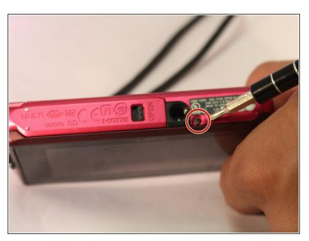
Using a Phillips #00 screwdriver remove one black 2 2/5mm screw near the tripod slot on the bottom of the casing.
