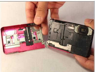
Remove the front casing of the device.
