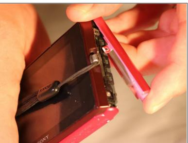
Pull the edge-casing off of the camera.
