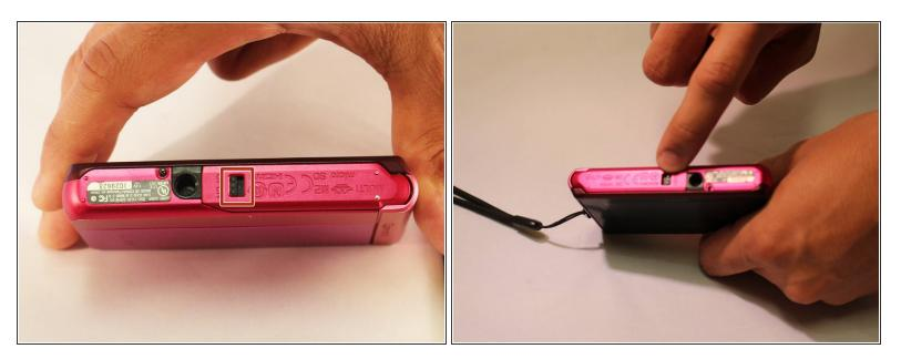
Using your finger, slide the release catch to unlock the battery/memory card cover.
