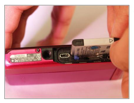
Remove the battery from the device.
