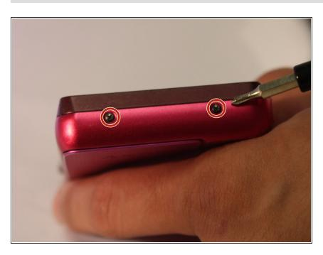
Using a Phillips #00 screwdriver remove the two 2 2/5mm black screws from the side of the camera opposite of the wrist strap
