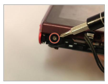
Using a Phillips #00 screwdriver, remove one 2 1/2mm screw located near the wrist strap.
