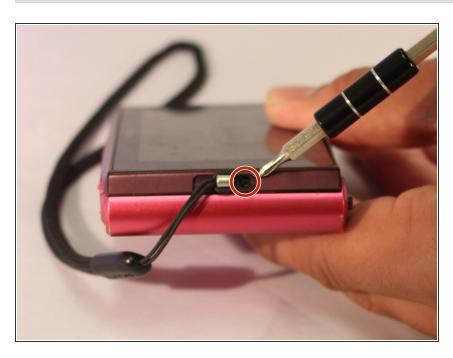
Using a Phillips #00 screwdriver, remove one black 2 2/5mm screw that is located next to the wrist band loop.
