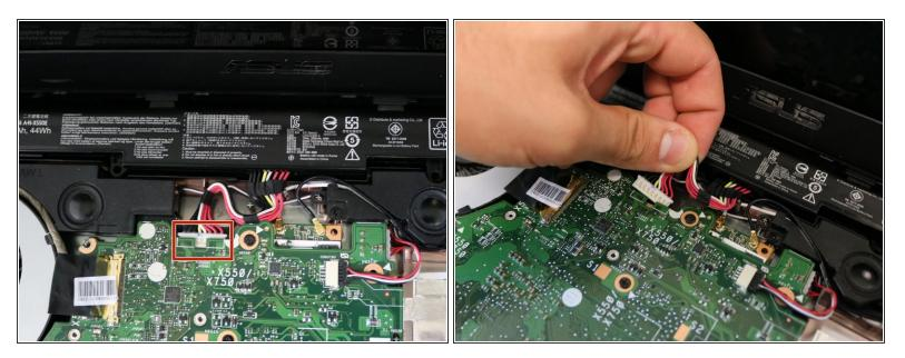
Disconnect the multi-wire battery plug from the motherboard.
