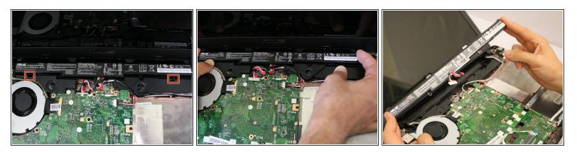
• Pull the two tabs holding the battery in place and lift the battery up. It should remove easily.
