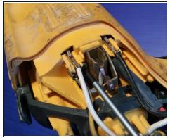
remove 1 torx ('t9) screw to remove the brush head.
