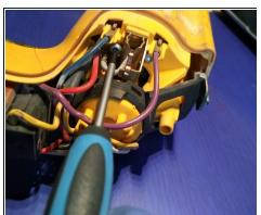
• remove the 2 swal torx (t9) screws, holding the brush head.
