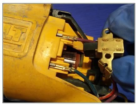
when replacing: push the brush in the head; click the wire on the right place and put it back. sometimes you will need to push the brush in place.
