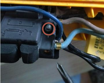
• remove the 2 small screws holding the brown and blue powerwires.
