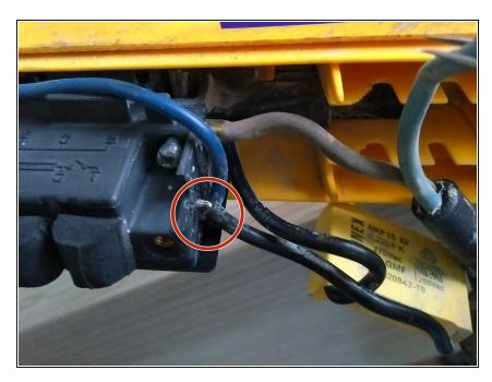
check fot bad connections. ( in this case you will see one bad connection from the condensator )
