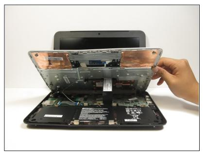
Lift the bottom of the keyboard assembly to reveal the internal components of the device.
