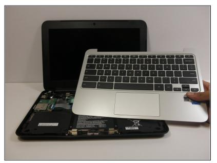
Remove the keyboard assembly by lifting it off the laptop base.
