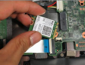
• Gently slide out the Wi-Fi card away from the motherboard by gripping the edges with your thumb and index finger.
