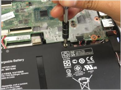
Remove the six 4mm Phillips #1 screws.
