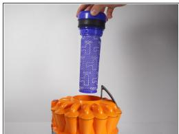
Remove the purple pre-filter by pulling it up and out of the bin.
