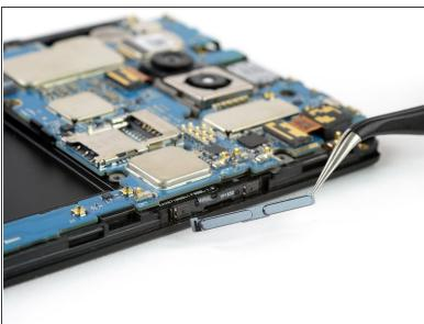
Use the flat end of a spudger to slide the volume button out of its bracket and remove it.
