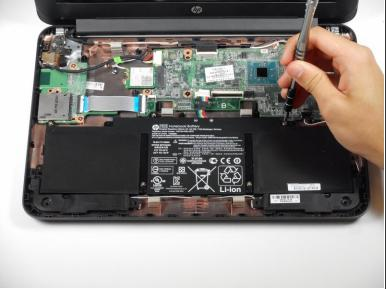
• Remove the six 4 mm Phillips #00 screws located along the perimeter of the battery.
