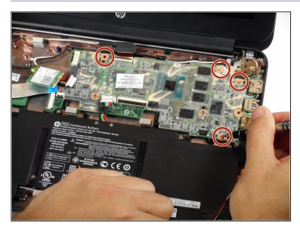
• Remove the four perimeter Phillips #00 6mm screws.
