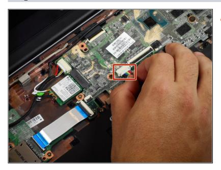
Gently pull the battery's rainbow-colored, bundled cable out of its socket.
