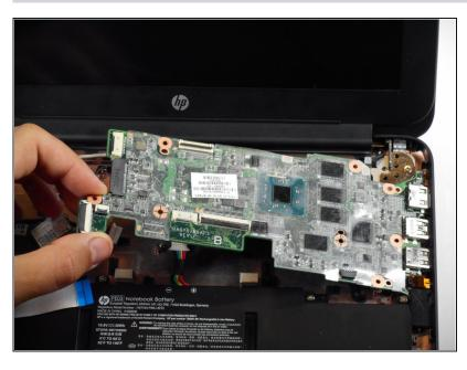
• Gently slide the motherboard to the left and away from the external ports on the right and then pull it up and out of the laptop.
