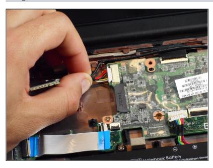
• Gently pull the bundled cable that connects the charging port to the motherboard out of its connector on the motherboard.
