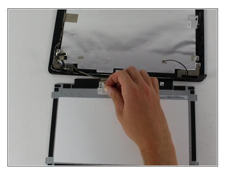
Peel the tape that holds the cable connector in place and slide the connector out.
