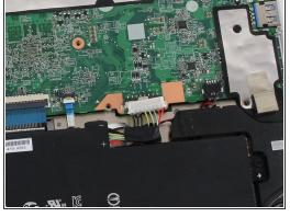
To disconnect the battery, pinch the multi-color bundle cable with your thumb and forefinger and pull directly back.
