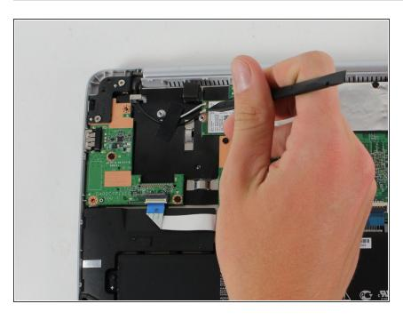
Use a spudger to disconnect the white and black antenna cables connected to the wireless card.
