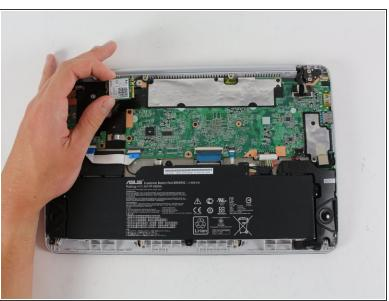
Grab the wireless card between your thumb and index finger and pull directly away from the motherboard.
