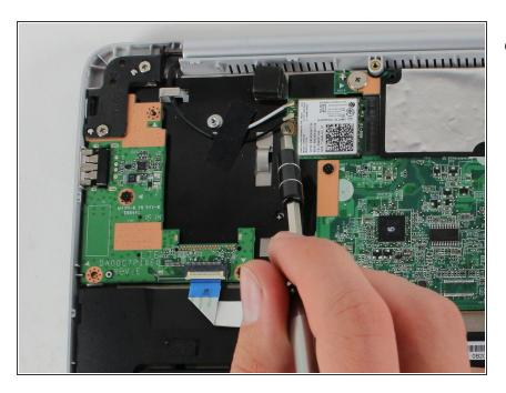
Remove the silver 2.8 mm Phillips #0 screw from the wireless card.
