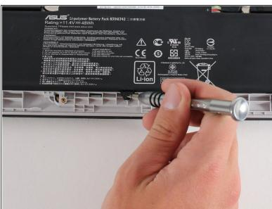
Remove the four 4.7 mm Phillips #0 screws that secure the battery to the Chromebook.
