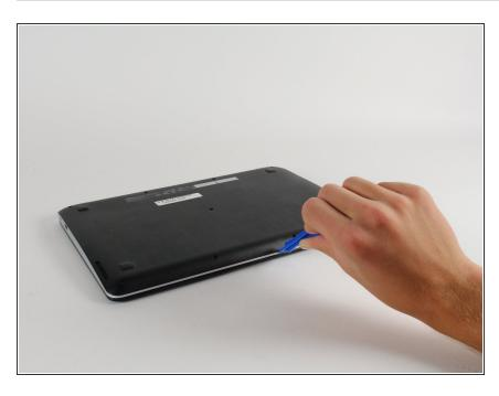
Use the plastic opening tool to gently work around the edge of the Chromebook until the back panel starts to lift off.
