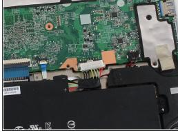
To disconnect the battery, pinch the multi-color bundle cable with your thumb and forefinger and pull directly back.
