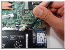
Unplug the black connector attached to the motherboard at the top right of the battery by using a spudger to push the two L-shaped indentations towards the battery.
