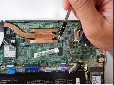
Remove the four 3.7 mm screws with a Phillips #0 screwdriver.
