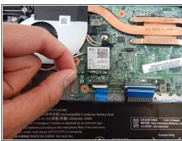
Disconnect the two white and black wires by holding close to the metal snap-on caps and pulling upwards.
