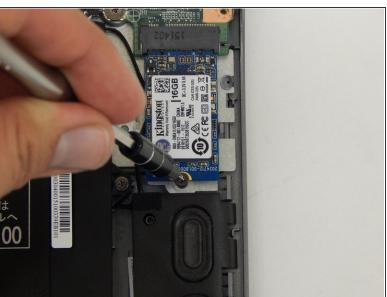
Remove the 3.75 mm screw with a Phillips #0 screwdriver.
