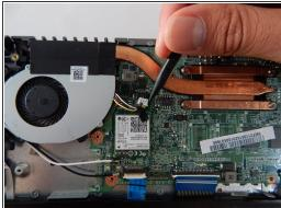
Unplug the white connector attached to the right of the fan with the spudger by applying force towards the battery on the two L-shaped indentations.
