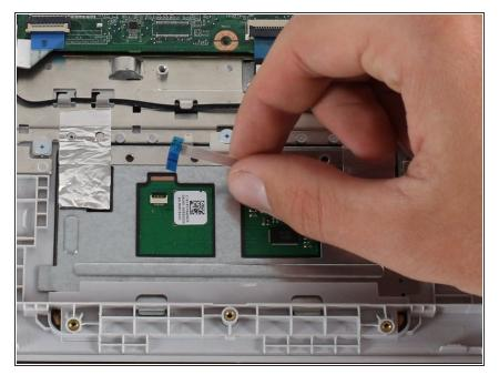
• Gently remove the adhesive on the touch pad ribbon cable.
