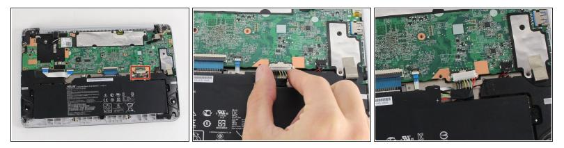
To disconnect the battery, pinch the multi-color bundle cable with your thumb and forefinger and pull directly back.
