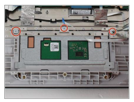
Remove the three 1.8 mm Phillips #00 screws.
