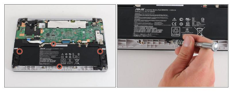
• Remove the four 4.7 mm Phillips #0 screws that secure the battery to the Chromebook.
