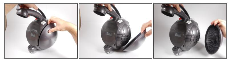
Pull the wheel away from the main body of the device.
