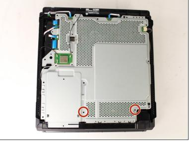
Use a T8 Torx security screwdriver to remove the two 10mm silver screws from the metal plate.
