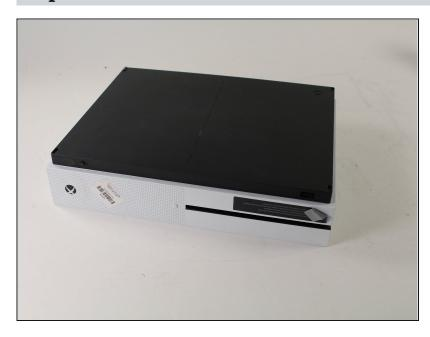
Flip the Xbox One S so that the bottom of the case is facing upward.
