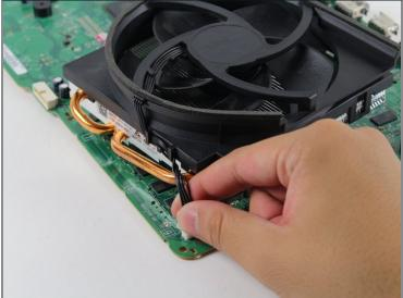
Detach the fan/heatsink from the board by gently pulling up on the plastic white connectors.
