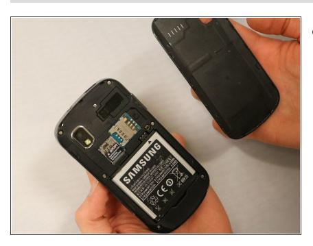
Remove the back cover with the spudger.
