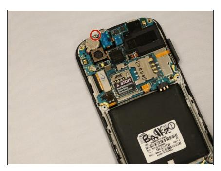
Remove the Phillips #000 screw that binds the auxiliary port.
