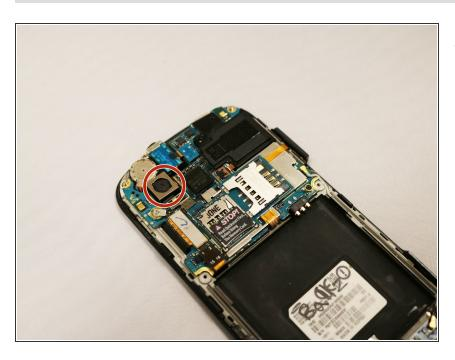
Indicate the camera, and carefully disconnect it with the spudger.
