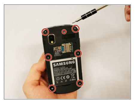
Using the PH000 screwdriver, remove the 7 screws in the back of the device
