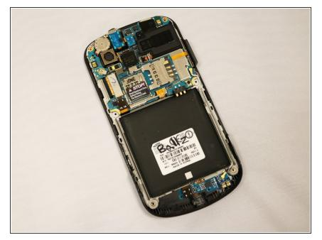
• Use the spudger to open and remove the rear panel.
