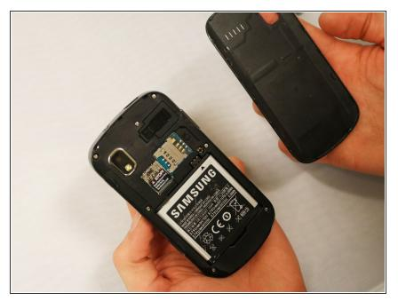
• Remove the back cover and take the battery out.
