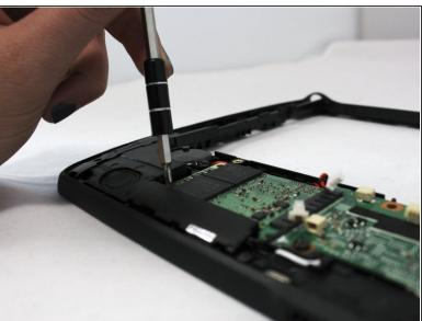
Remove the 3mm Phillips #0 screw from the SSD drive which is located above the speaker and to the left of the motherboard.
