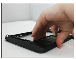
• Using your hands or the blue plastic opening tool, go along the edges of the frame and unsnap the screen from the middle frame.
