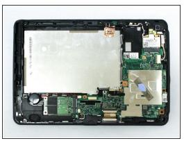
Pull up on the black tab located at the top of the battery to remove the battery from the device.
