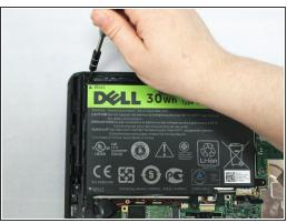
• Remove the three 6mm Phillips #0 screws attaching the battery.
