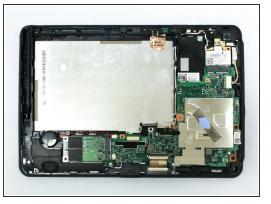
Pull up on the black tab located at the top of the battery to remove the battery from the device.
