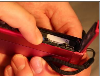
Push the battery eject lever to free the battery.
