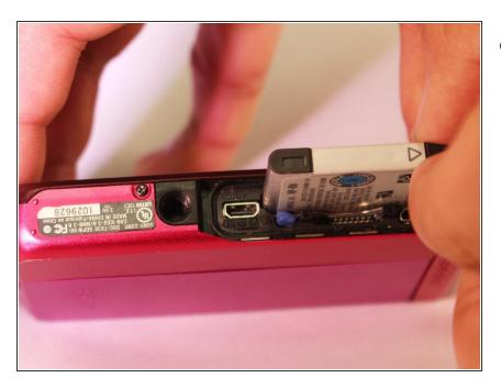
Remove the battery from the device.
