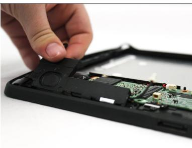
• Using the plastic opening tool, pry the speaker up to remove it from the device.
