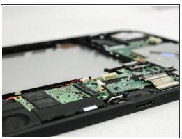
Using your hands or a plastic opening tool, disconnect the white speaker connector from its socket near the bottom of the motherboard.
