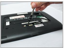
Using a Phillips #0 screwdriver, remove the four 6mm screws attaching the inside panel to the device.
