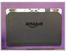
Start by removing the plastic cover to the speakers and webcam. I used a couple of spudgers, but you can also see the exploded version from the product video still I included, as well. Take your time, this is probably the most patient part of the whole repair.
