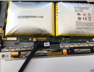
These are both <u>ZIF connectors</u>, meaning they use a friction flap to hold them in place. Carefully lift the flap, and disconnect the ribbon cabling for both cables.
