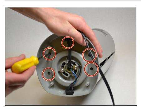
Remove the five screws that can be seen by aligning the base and the fan.
