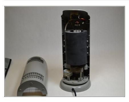
Remove the back casing by pulling it away from the front casing.
