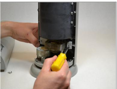
Remove the two screws attaching the motor to the front casing.
