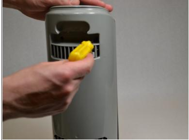
Stand the fan upright. Locate and remove the two screws near the top.
