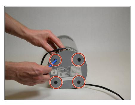
Using a plastic opening tool, remove the four small foam pieces on the bottom of the fan.
