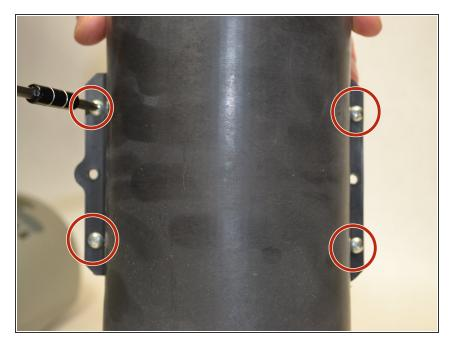
Remove the four remain screws holding the air filter casing together
