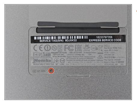
• Remove the single Phillips screw hidden beneath the flap.
