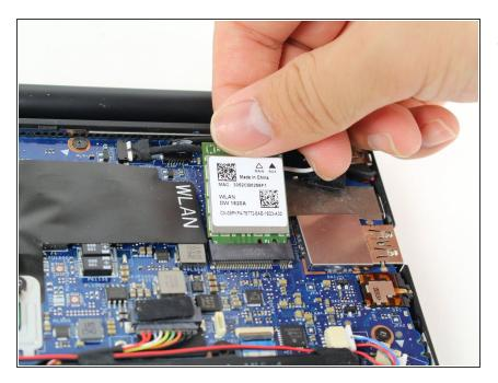
• Pull the wi-fi card straight out of its socket.
