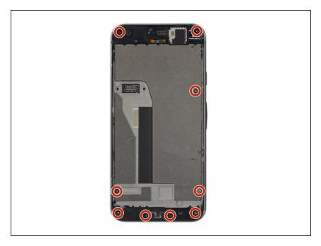
Use a T5 Torx driver to remove the nine 3.5 mm screws securing the midframe.
