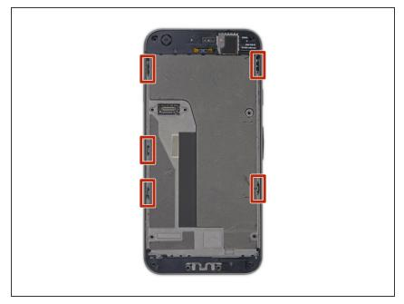
The midframe is held tightly in place by five clips. To release these clips, apply inward pressure with an opening tool as shown in the steps below.
