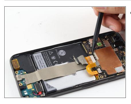
Use a spudger to disconnect the charging port ribbon cable from the motherboard.
