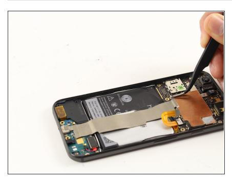
Use tweezers to lift up the adhesive strip at the top of the battery, and peel it back to expose the connector underneath.
