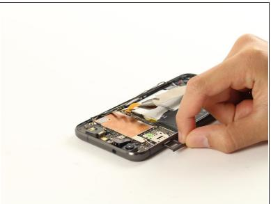
Use a SIM ejection tool to remove the SIM card tray located at the top left of the device.
