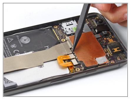
• Use a spudger to pry up the battery ribbon cable, disconnecting it from the motherboard.
