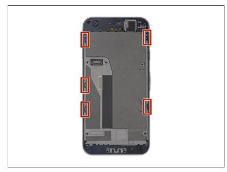
The midframe is held tightly in place by five clips. To release these clips, apply inward pressure with an opening tool as shown in the steps below.
