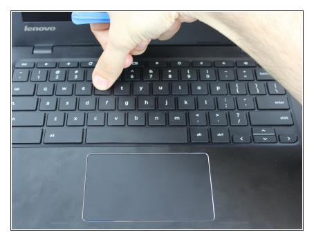
Gently put new key back into position by pressing down on they keycap until it snaps back in place.
