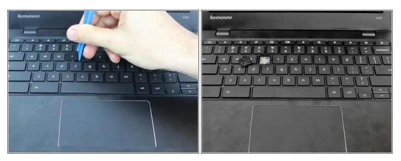
• Use the plastic opening tool to remove the key by prying it up from underneath.
