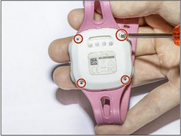
Use the Torx 5 Screwdriver to remove all four 1.1 mm screws on the back of the watch.
