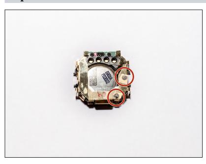
Secure the two springs with two small pieces of scotch tape to ensure the springs do not fall out.
