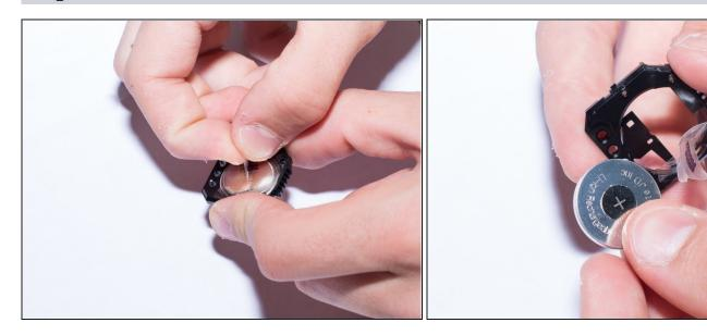
• Separate the clear tape attached to the battery.
