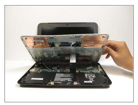
Lift the bottom of the keyboard assembly to reveal the internal components of the device.
