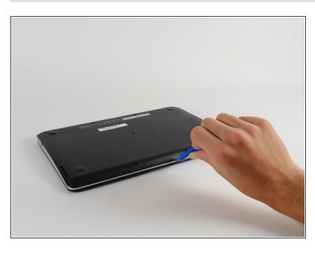
Use the plastic opening tool to gently work around the edge of the Chromebook until the back panel starts to lift off.
