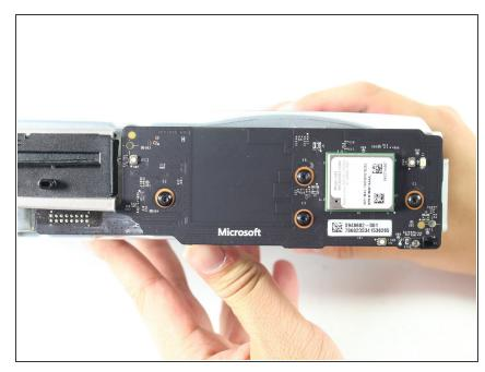
The IR blaster can be identified on one of the sides of the interior case. It will be next to the disc drive and near the fan.
